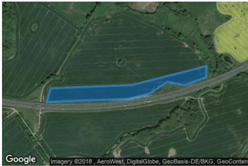
**Name:** TF 3**Axis tracking:** Fixed (no rotation)**Tilt:** 20.0 deg**Orientation:** 180.0 deg**Rated power:** -**Panel material:** Light textured glass with AR coating**Vary reflectivity with sun position?** Yes**Correlate slope error with surface type?** Yes**Slope error:** 9.16 mrad
