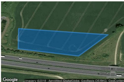
**Name:** TF 2**Axis tracking:** Fixed (no rotation)**Tilt:** 20.0 deg**Orientation:** 180.0 deg**Rated power:** -**Panel material:** Light textured glass with AR coating**Vary reflectivity with sun position?** Yes**Correlate slope error with surface type?** Yes**Slope error:** 9.16 mrad
